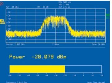
Power measurement of a 3GPP HSDPA signal.
