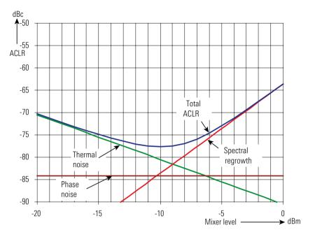
Dynamic range of the R&S<sup>®</sup>FSU for adjacent-channel power measurement on WCDMA signal without noise correction.
