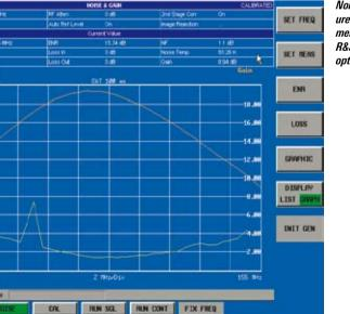
Noise figure measurement with the R&S<sup>®</sup>FS-K30 option.
