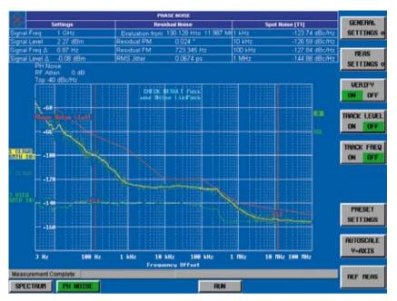
Phase noise measurement with the R&S®FS-K40 application firmware.
