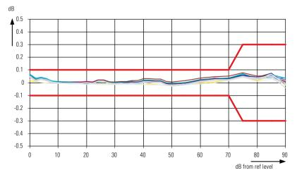
Display linearity at ≤100 kHz resolution bandwidth (measured on 30 instruments).
