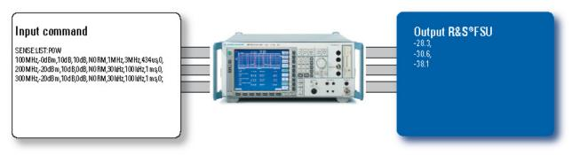
Remote control of the R&S<sup>®</sup>FSU via IEC/IEEE bus in list mode cuts down on measurement time.
